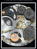
The dial side of the movement shows a multiplicity of solarand civil-time functions powered by separate gear trains.
